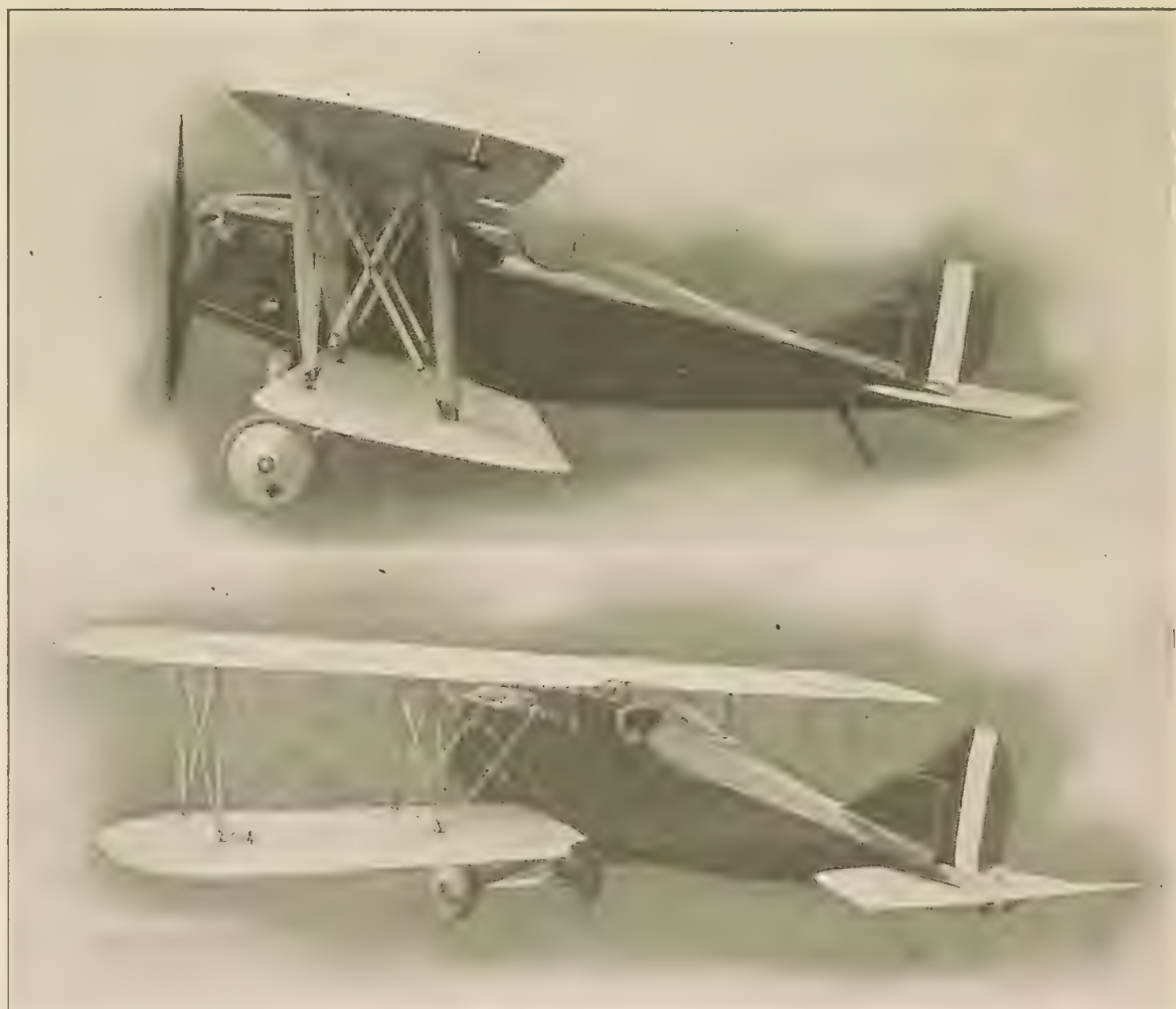
Ordnance Engineering Corporation type D single-seater fighter, with 300 hp. Hispano-Suiza motor. Span, 30 ft. Overall length, 21 ft. 6 in. Height, 8 ft. 3 in. Total weight, with full military load, 2355 lb. Fuel and oil for three hours' flight under full power. High speed, 157 m.p.h. Climb to 10,000 ft. in 6 min. 35 sec. The two synchronized guns are completely enclosed, yet readily accessible to the pilot. Equipment includes oxygen tank and parachute
